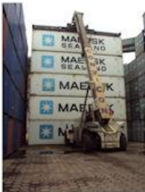
Figura 23 – Reach Stacker com Container
