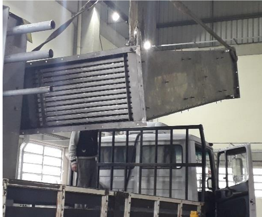
Heat recovery section with pillow plates.
