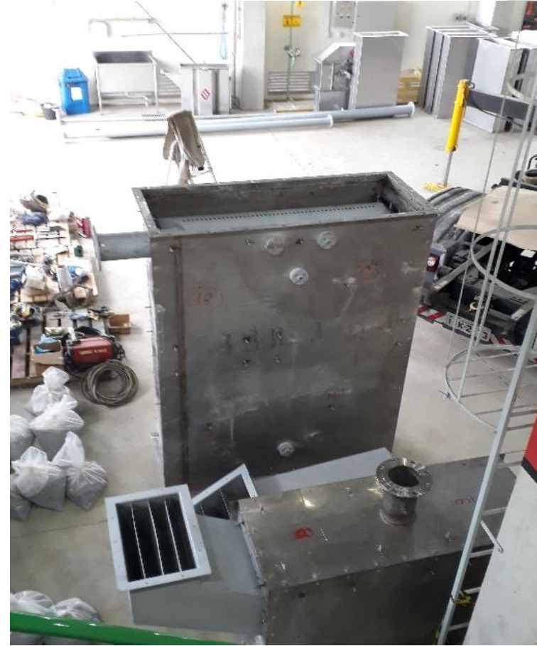
Adsorption section with flue gas distribution tube.
