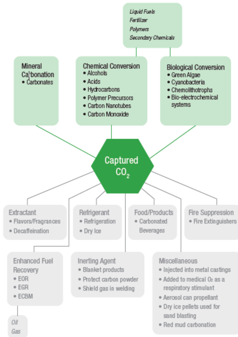
Figure 3.8. CO 2 utilisation pathways. Source: Gaseous Carbon Waste Streams Utilization: Status and Research Needs, National Academies of Sciences, Engineering, and Medicine (NASEM), 2019
