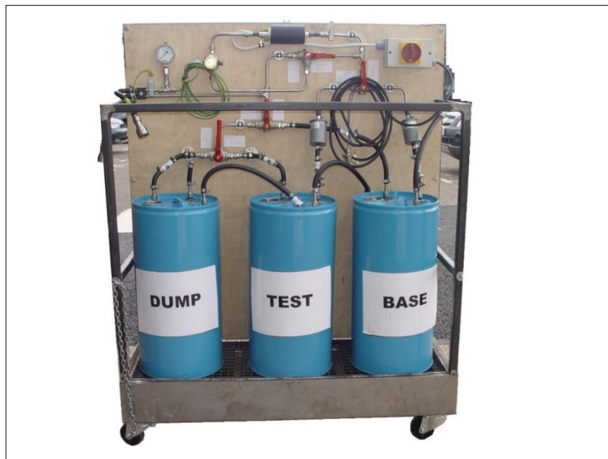
Figure 3 Fuel Changeover Rig
