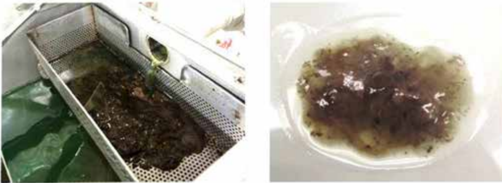
Figure DF - 37: Examples of Microbial Growth in B5
