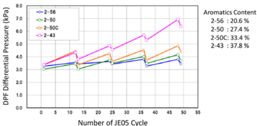
Figure DF - 29: Influence of Total Aromatics Content on DPF Differential Pressure
