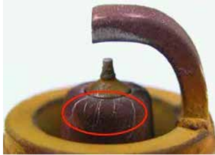
Figure G-19: Catalyst Thermal Damage by Misfiring of Spark Plugs Coated in Iron (UAE market, mileage 50,000km)
