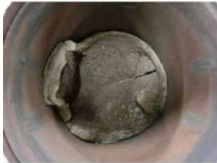
Figure G-19: Catalyst Thermal Damage by Misfiring of Spark Plugs Coated in Iron (UAE market, mileage 50,000km)
