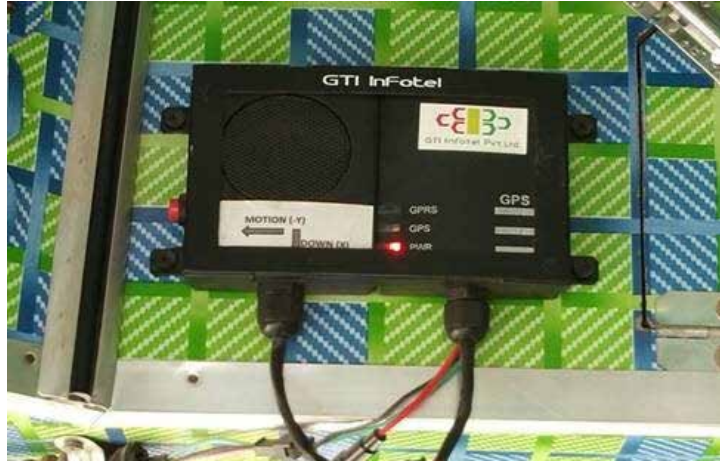
VTS VMU (vehicle mounted unit) mounted on an LPG Truck (IOC)
