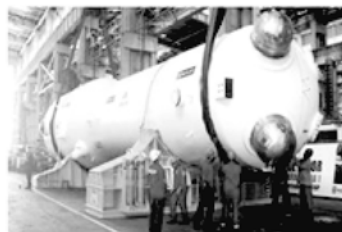
Geradores de Vapor substitutos para a usina nuclear Angra 1 Replacement Steam Generators for the Angra 1 nuclear power plant
