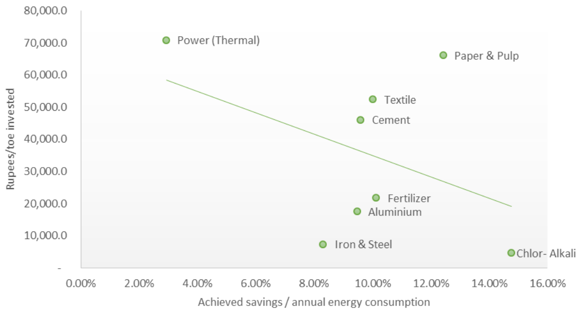
Figure 1 - Investment costs per toe vs the ratio of actual achieved savings over actual annual energy consumption. Ricardo analysis.
