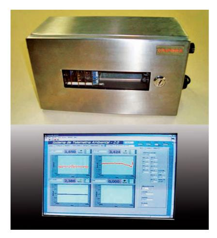
Above is the Caipora recorder, which stores the environment data and transmits them to a computer through telemetry.
