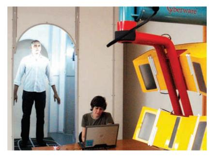
Tridimensional laser scanner image captures human image for use in an ergonomics project addressed to the oil and gas industry.
