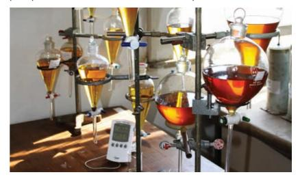
Biofuels: storage tests at the Laboratory of Corrosion and Protection.
