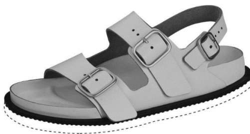
Example of contextual element (unclaimed), represented by dashed lines in a rendered industrial design.
