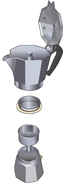
Example of exploded view representation
