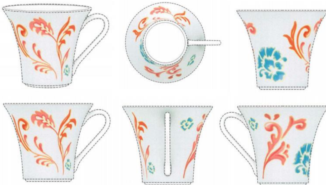
Example of ornament applied to a tridimensional product in which six views are necessary to fully claim the industrial design of the ornament (DI7102778)
