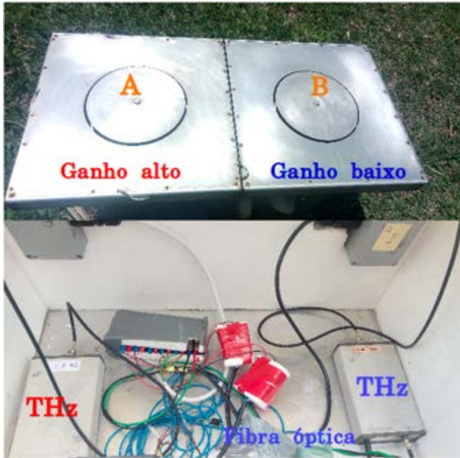
Figure 4.5 - Electric field sensor that shows the internal and external part of the sensor.
