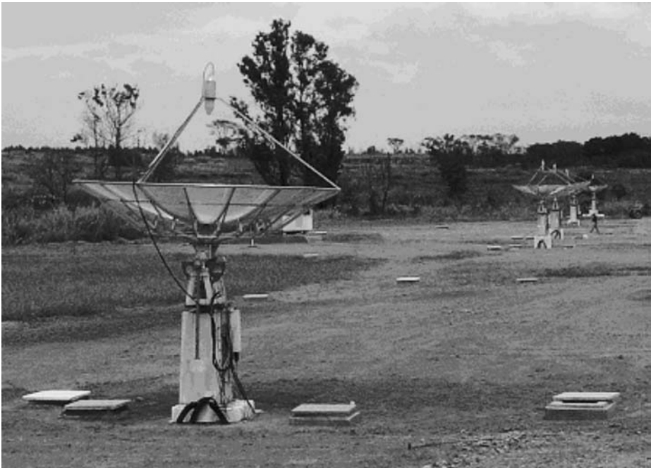
Figure 1 Phase-I of the BDA at the INPE campus in Cachoeira Paulista (longitude 45^{\circ}0'20'' W, latitude 22^{\circ}41'19'' S). The array is in the E–W direction and the longest baseline length is 216 m. The antenna (A5) in the foreground is the East end of the array.
