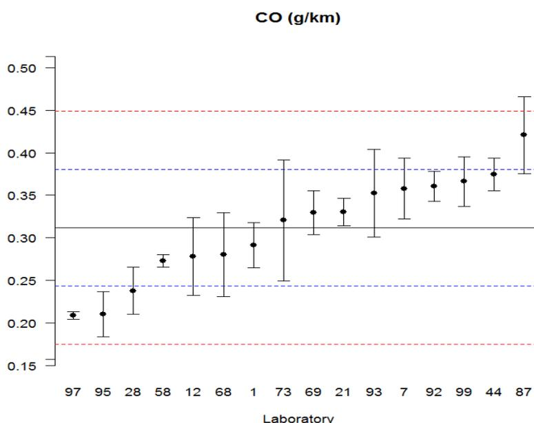
Figure 01 – Scatter plot of the results for CO determination
