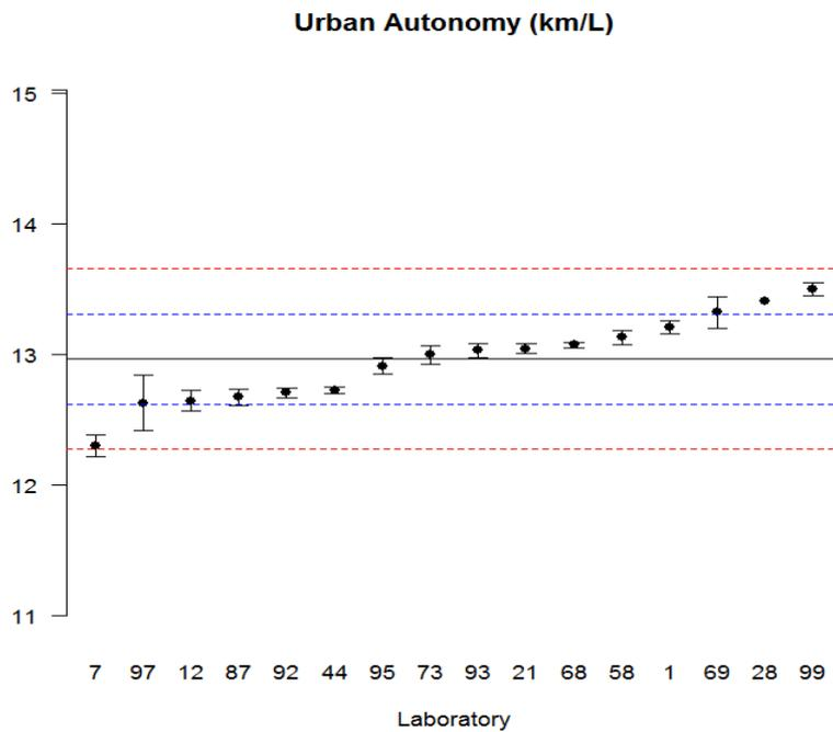
Figure 07 – Scatter plot of the results for Urban Autonomy determination
