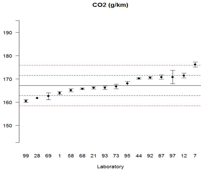
Figure 02 – Scatter plot of the results for CO<sub>2</sub> determination
