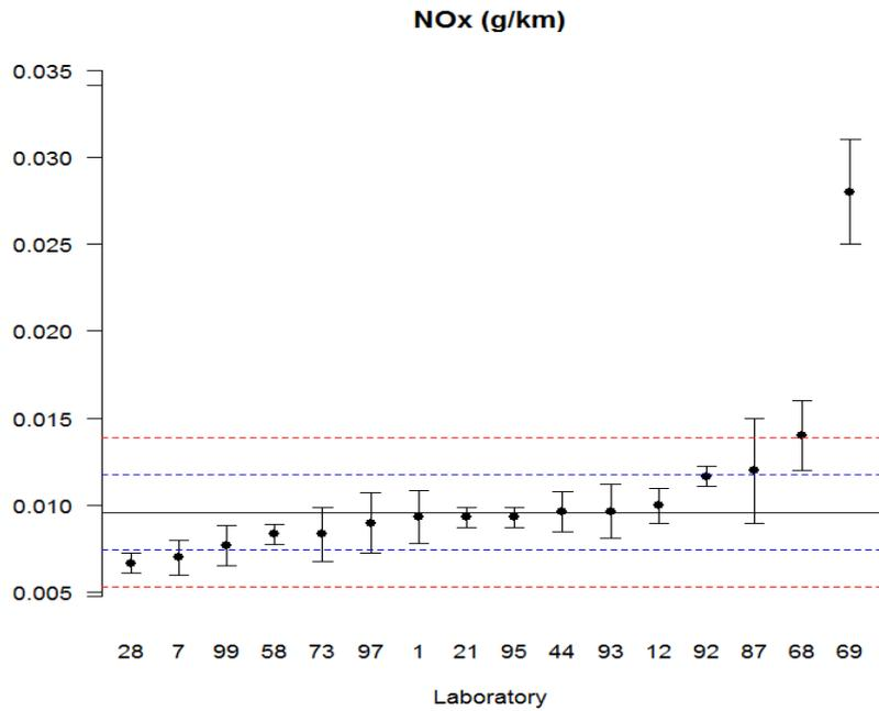
Figure 05 – Scatter plot of the results for NO<sub>x</sub> determination
