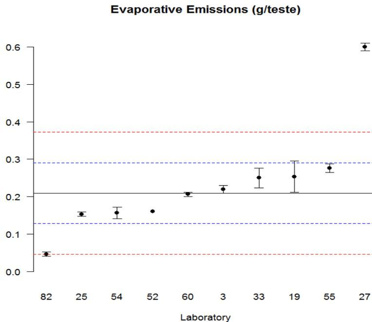
Figura 09 – Scatter plot of the results for Evaporative emissions hot phase
