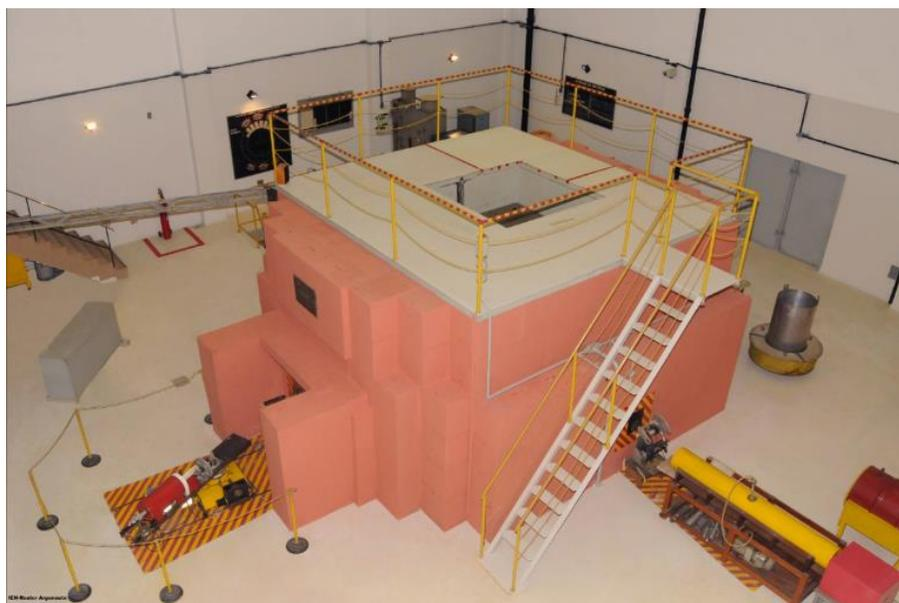
Figura 17: Reator Argonauta
