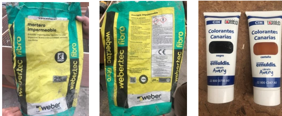
Figure 6. Example of material that can be used in the manufacture of artificial rock walls for Lear's Macaws. Left and center: mortar with waterproofing. Right: mortar dyes (Photos: Loro Parque Fundación).
