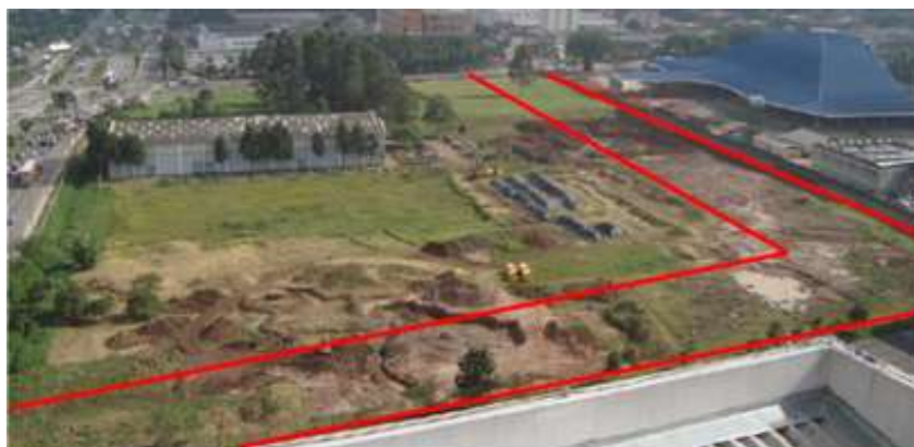
Figure F.7 - USIM - the red range represents the decontaminated area - 18,400 m 2
