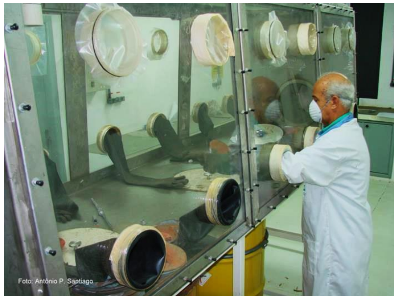
Figure H.3 – Glove box equipped to dismantle lightning rods
