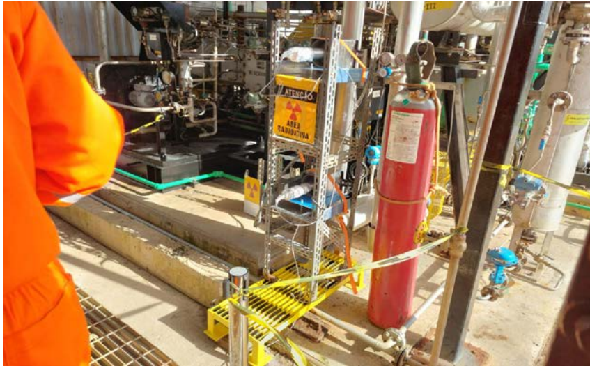
(Photo: Scintillator detectors installed to measure flow speed in a natural gas processing plant in Aracaju, Brazil. Source: IEN/CNEN)
