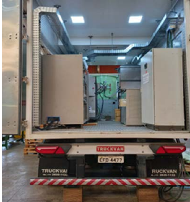
(Photo: Rear section of the mobile unit with electron beam accelerator. Source: IPEN/CNEN)
