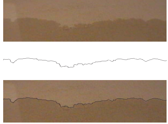
FIGURE 2. Image treatment of the air/liquid interface. The top panels shows the image captured from the digital camera, which was treated with ImageJ TM in order to obtain a single valued function, shown in the middle panel. The bottom image combines the single value function and the original image to compare the efficient of the procedure.
