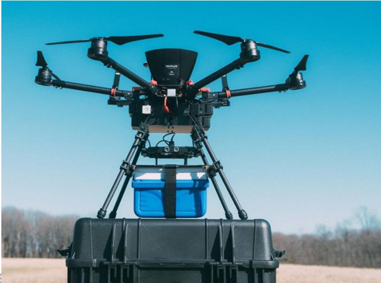
Johns Hopkins researchers attached a cooler packed with blood products to a S900-model drone.
