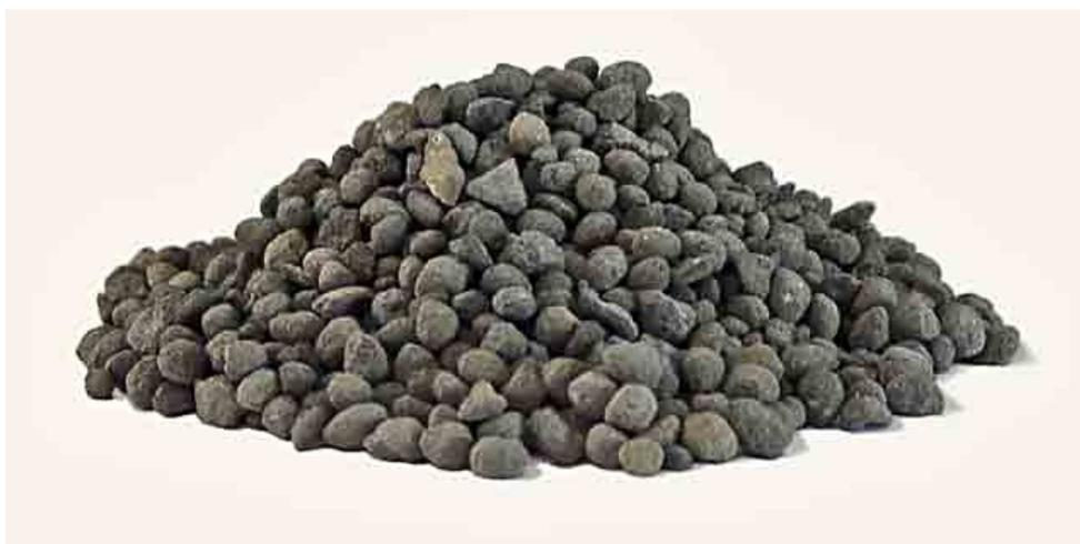
Figura 3.3: Clínquer de cimento Portland. FONTE: <http://www.cementkilns.co.uk/>
