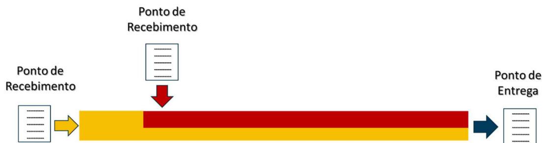
Image 7 - Schematic of the calculation of the chemical composition of the delivery points from the chromatographic data of the receiving points.
