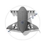
D = diameter of the smallest circle enclosing the projection of the eVTOL aircraft in a horizontal plane, while the aircraft is in takeoff or landing configuration, with rotor(s) spinning, if applicable.
