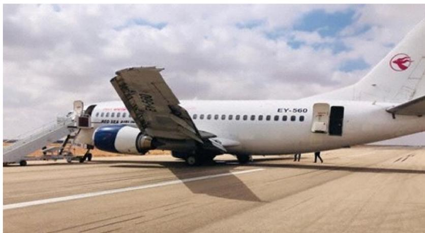
Accident: Djibouti B735 at Garowe on Dec 2nd 2020, touched down short of runway, gear collapse on roll out
