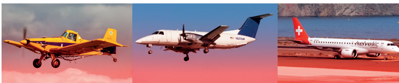
Figure 12: examples of aircraft – from left to right: piston-engine aircraft, turboprop aircraft and jet aircraft.
