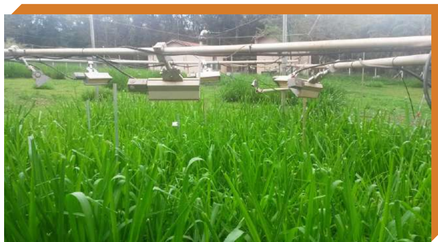
Figure 2: Detail of a portion of the T-FACE System (Temperature free-air controlled enhancement) for simulating global warming under field conditions.
